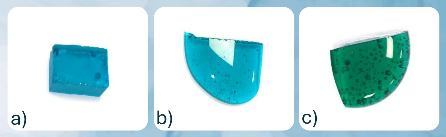
Comparison of glass samples with 5% Cu concentration, a) original glass b) treated glass at 700°C and 1 hour c) treated glass at 700°C and 10 hours – colour shift implies change of copper oxidation state with longer treatments
